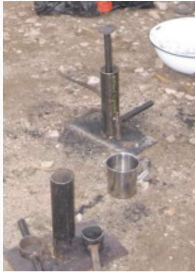
First Prototype $30 4-5 Briquettes a Minute
