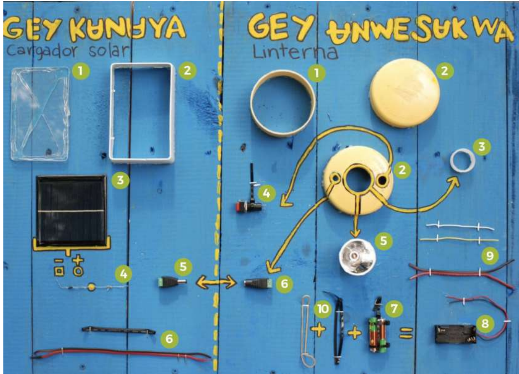
Solar-powered led-light and solar charger instructions.
