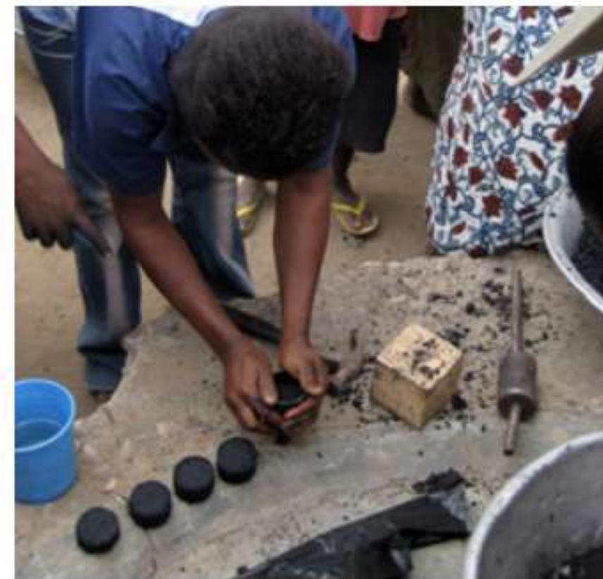
6. Pressing charcoal mixture into briquettes
