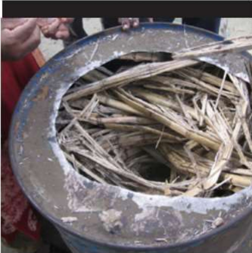
1. Placing bagasse in the oil drum
