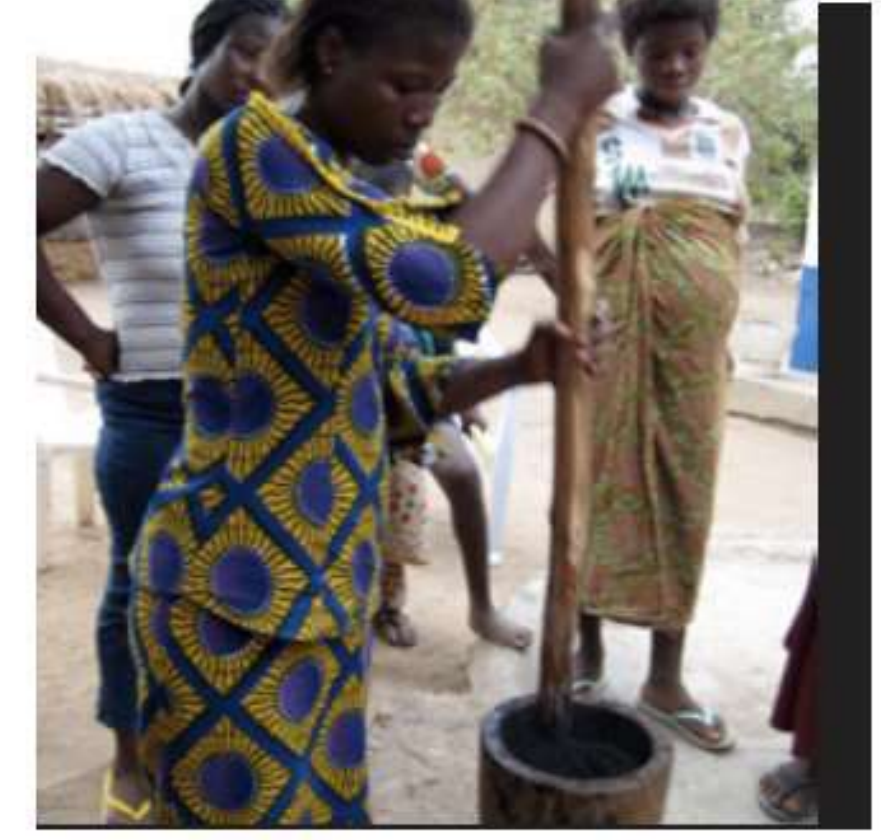
4. Crushing carbonized corn cobs into a powder
