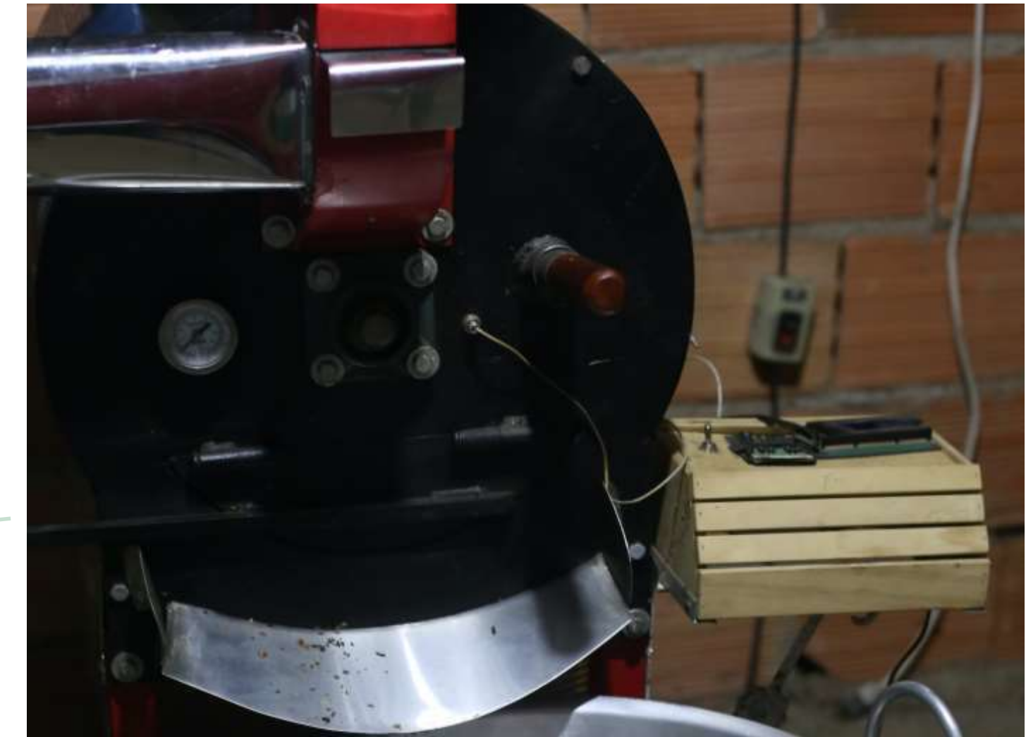
Arduino-based roasting curves automatized system
