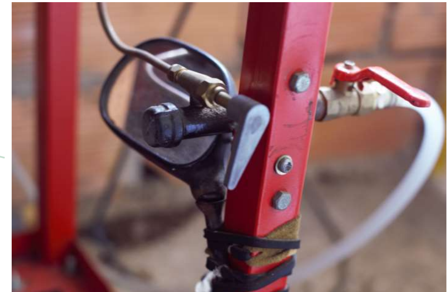
Car rearviewmirror used to track coffee beans color shading inside the roasting drum
