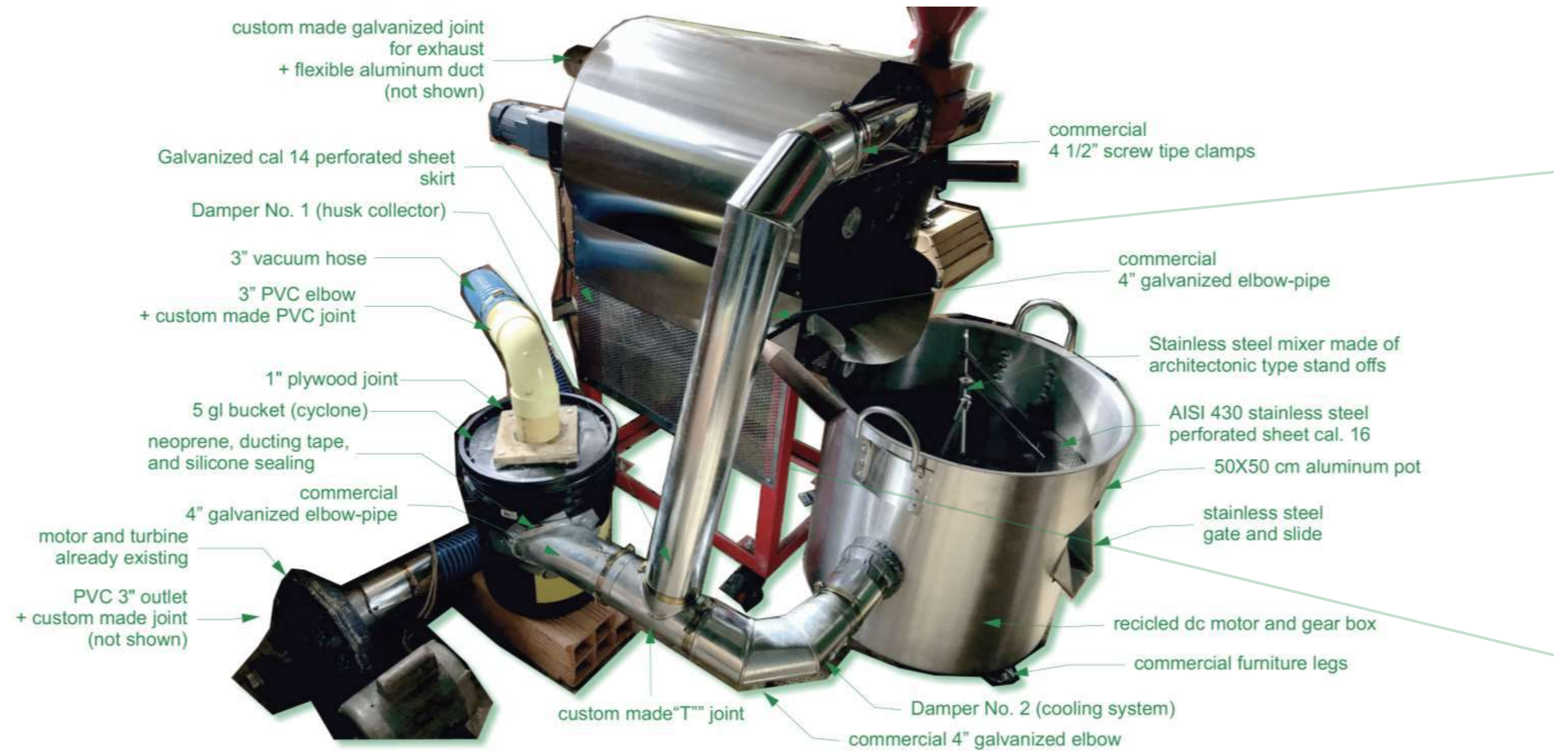
Coffee roaster with coffee cooling and ventilation systems.
