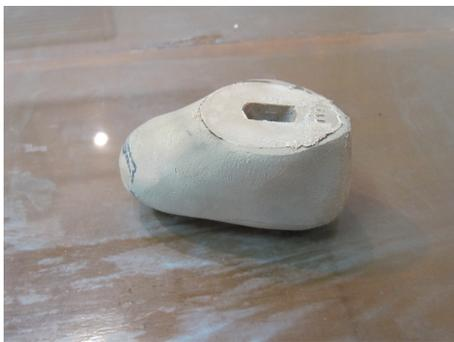
Figure 16: Prototype 2 was a shorter foot that would be easier to pull out of the mud.
