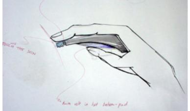
Figure 13 One of the concepts: A shaving device which allows your fingertips to immediately feel the effect. By feeling every move, the shaver may build a memory of the shaving actions on his skin because it is 'in his fingertips'.
