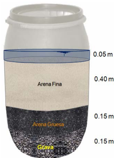
Figure 4. Filter Bed Structure
